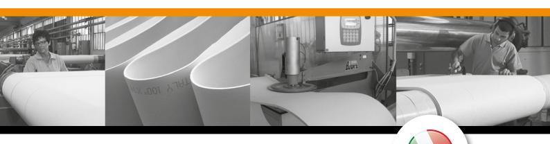
**ITB** seamless pasting belts are heat set at high temperature under remarkable stretching load: their dimensional stability is therefore excellent throughout their service life.
